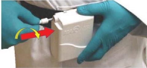
7. Using a slight twist, connect power cord to battery.
